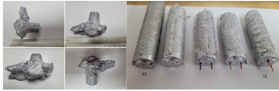
Figure 5. Left- partial rod cast during zero-g, right-rods cast in 1G,
